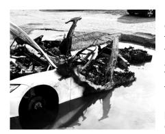
Lithium-ion batteries can be found in all types of devices, tools, electric vehicles, and energy storage. When these batteries fail in thermal runaway, they can produce fire and explosion hazards.
